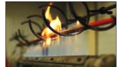
Fig 5 - Enhanced cable undergoing testing to requirements of BS6387 Category C to test resistance to fire alone
